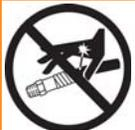
Do not install shutoffs downstream of the PRESSURE RELIEF/SPRAY valve outlets (BA, BB). The valves function as overpressure relief valves when set to SPRAY. Lines must be open so valves can automatically relieve pressure when machine is operating.
