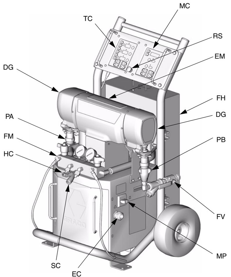
**FIG. 3: Component Identification**
