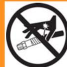
Read warnings, page 5. Thermal expansion can cause overpressurization, resulting in equipment rupture and serious injury, including fluid injection. Do not pressurize system when preheating hose.
