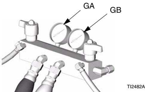
**9.** Open gun fluid manifold valves A and B.
